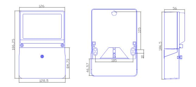
Meter external dimensions (unit: mm)
